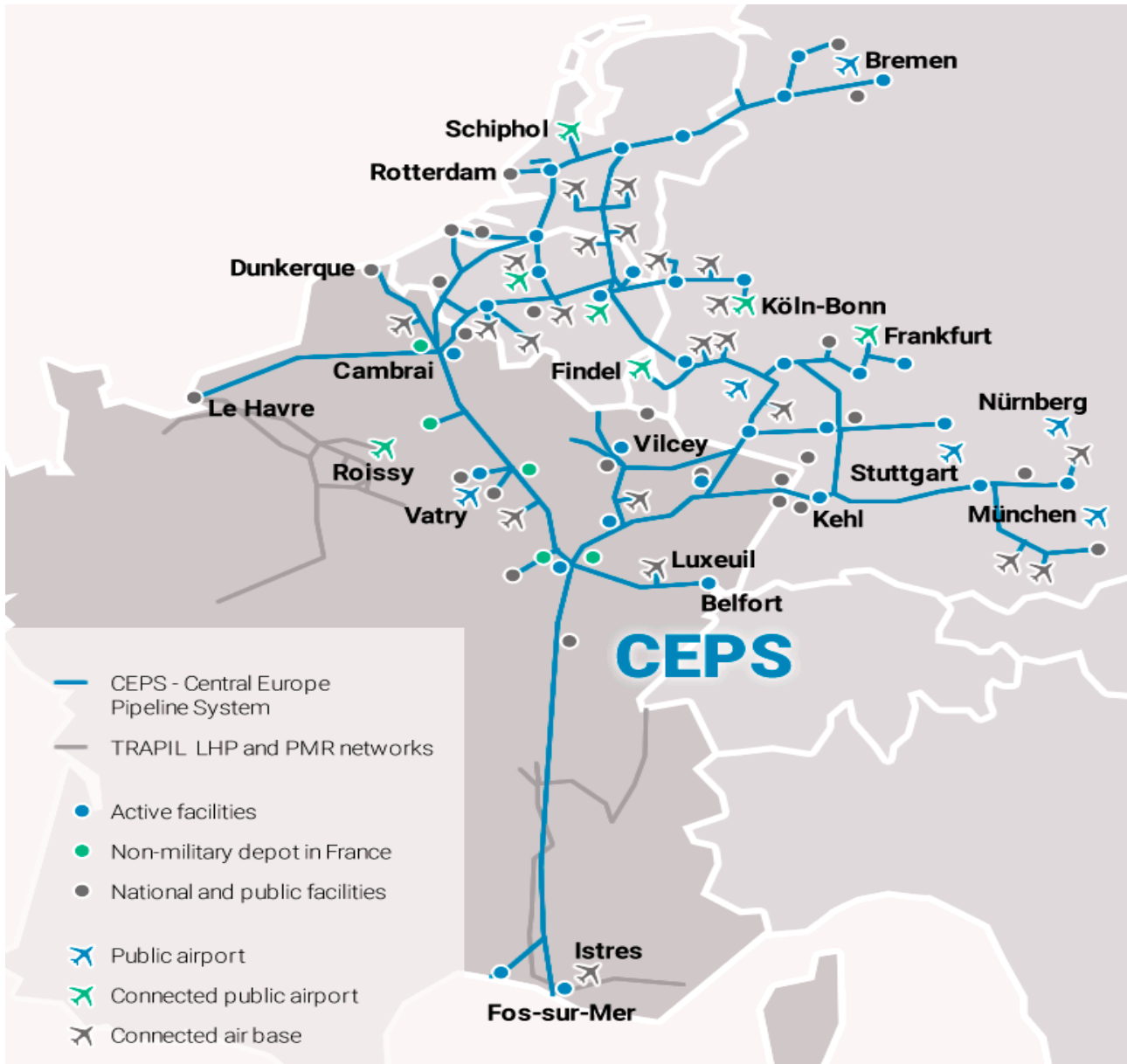
Figure 3: The pipeline network of NATO CEPS (Central European Pipeline System) for kerosene in Western Europe. Commercial airports connected to the CEPS are identified by a green icon [CIM and CCMP 2024, the CEPS network]
