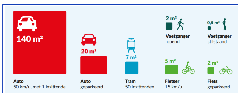
Figure 35: Use of space by modes of transport and per passenger. Space taken for mODiNg tram is absent in this figure. 51
